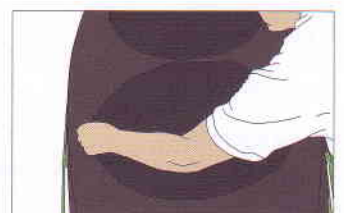
7. The cap and skirt is installed through the spraycover channel.
