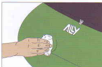
4. To enhance the bond, wash both the marked canoe skin bond area and the attach-loop bond area with acetone. A simple cotton cloth may be used.
