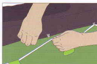
6. Thread the bungee cord through the attach loops and secure the two ends by tying them together. You can now hook the spraycover on to the bungee cord all the way around.
